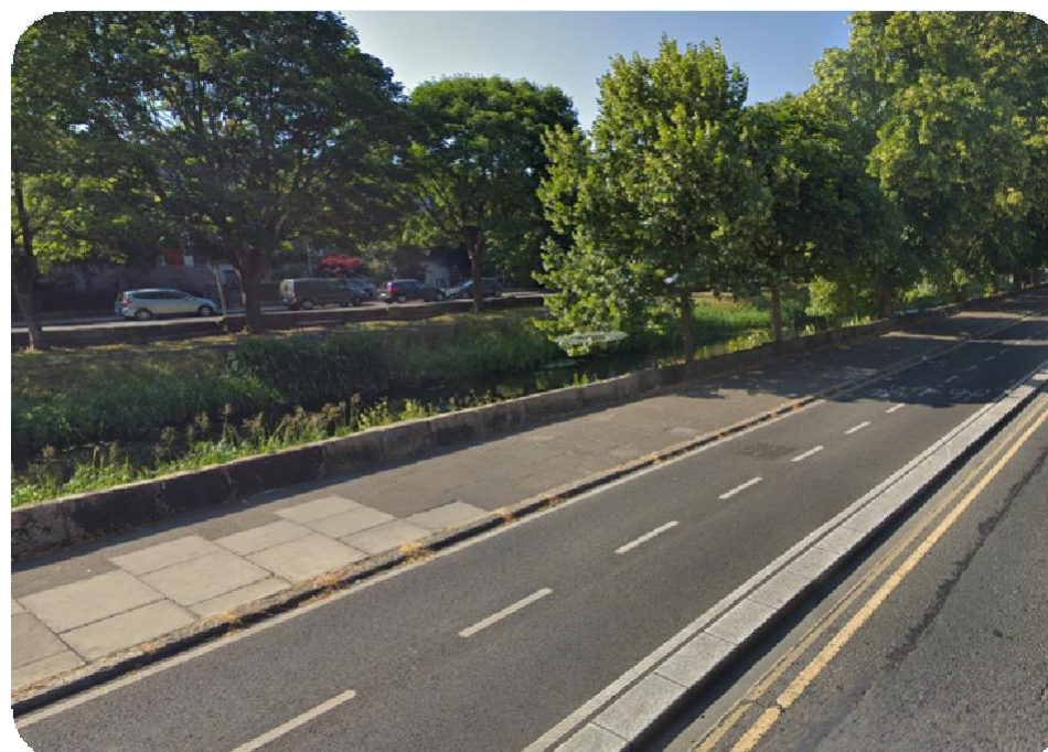
Figure 8: Preferred CBC Cycle facility segregation (example shows a two-way cycle track)
